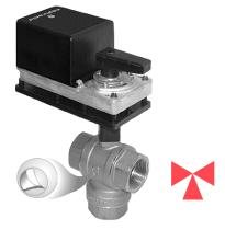
The **Contoured Port Series** are actuated **Ball Valves** that can provide digital or analog control of hot and chilled water systems containing up to 50% glycol. Each unit is comprised of a rotary actuator and linkage assembly coupled to a valve body that offers positive close off and low torque. The Contoured Port Ball, incorporates an integral permanently attached glass filled polymer to achieve a wide range of Cv's by offering a variety of orifices.
